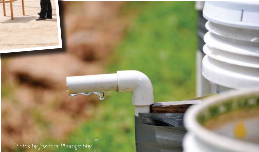
Top to bottom: San Damian is nestled high on the hillside; Chuck Firestone leads the mud-brick cook stove workshop; Originally contaminated with worms and bacteria, clean water comes from the biosand filters.
